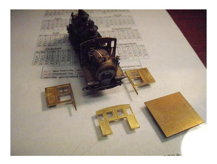
The next step(s) were to re-solder all the sides and rear to the frame and each other. That was not the easiest as I only have two hands and with a soldering iron on one, I was quite handicapped. There are times we all will agree that having a Durga around would be most helpful.
