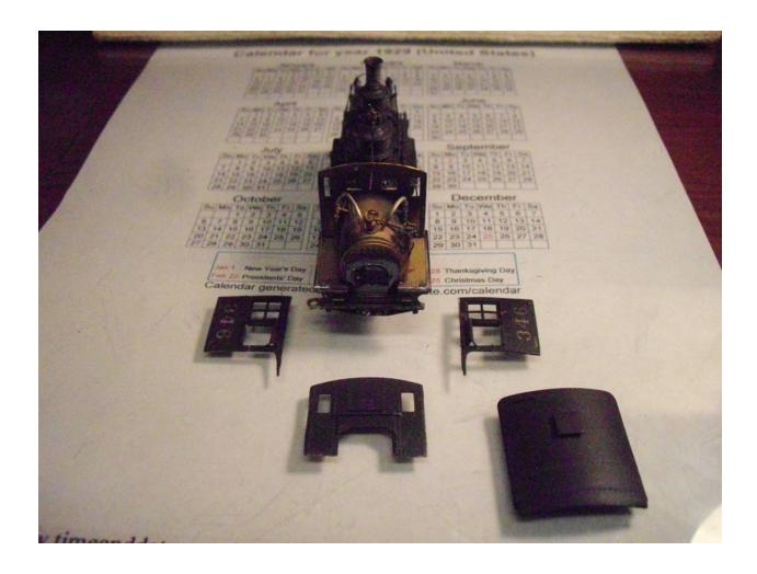
Now I was tasked with attempting to retro-fit the proper wooden cab to the frame. The biggest item of note was what cab to purchase. A Precision Scale Company 1920's era wooden cab fit the requirements and was procured. As it was laid out and fitted, all seemed to be going back together as intended; better yet. Notice here that I did leave the front wall intact. I decided that a solid reference point would be most desirable for this exercise.
