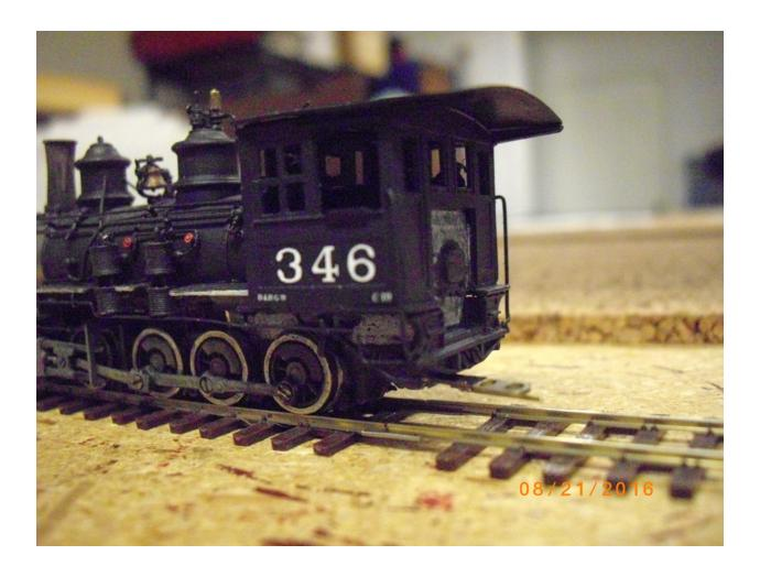
For the home stretch I removed the existing headlight and replaced it with a box headlight. That was an easy fix as it just about fell off and with a Dremel wire wheel plowing a road to the bare brass, the new headlight was soldered in place. Holes were drilled for wires and a LED was installed and are to be wired into the decoder. Note, the class lights have been replaced as well and with more LEDS inserted, they as well will be wired into the decoder.
